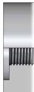
BSPP female port (spot-faced)
