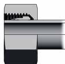
DIN cutting ring and nut on tube
