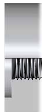
BSPP female port (spot-faced)
