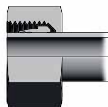
DIN cutting ring and nut on tube
