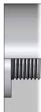
BSPP female port (spot-faced)
